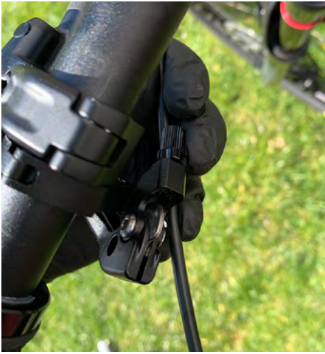
12. Line the outer cable up to the lever and determine the correct length required.
