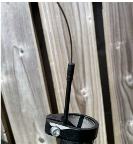
16. Install the inner cable into the outer from the seat tube end. You will end up with a lot of excess inner cable at the front of the bike.
