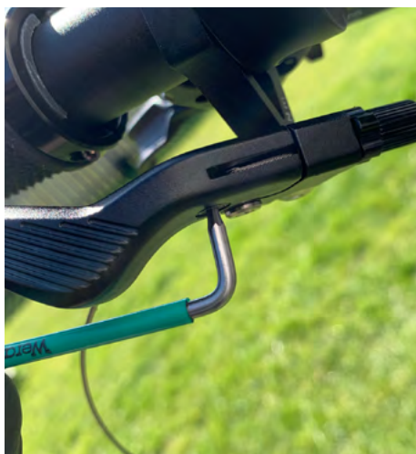
26. Pull the inner cable tight and tighten the grub screw.
