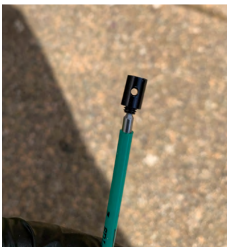
22. Take the small cable barrel and undo the grub screw a few turns until it is no longer blocking the hole.
