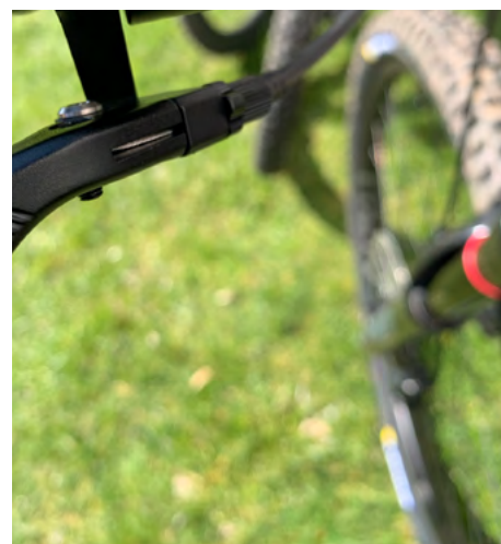
24. Route the inner cable through the lever and then through the barrel.
