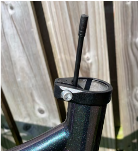
14. Remove the seatpost from the frame and push the outer cable back through the frame until the end is sticking out of the seat tube. You will likely end up with the outer cable down towards the downtube, this is completely normal at this stage.
