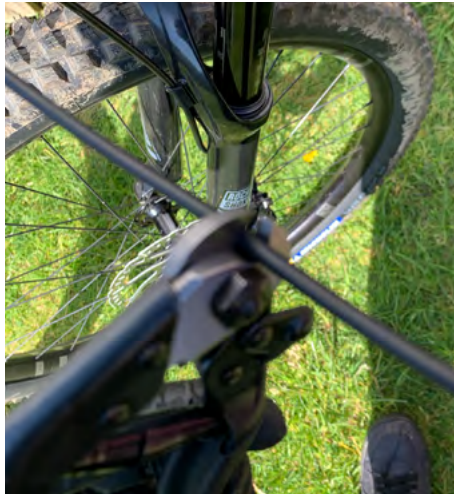
13. Double check cable routing is all correct then cut the outer cable to length and fit ferrule.
