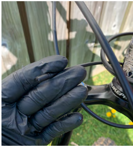
14. Remove the seatpost from the frame and push the outer cable back through the frame until the end is sticking out of the seat tube. You will likely end up with the outer cable down towards the downtube, this is completely normal at this stage.
