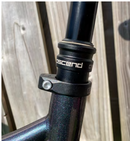
20. Insert seatpost to required depth using the measurement from step 6.
