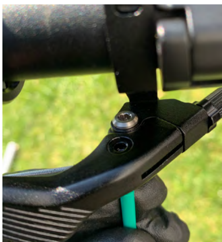
23. Move the lever to the closed position and then place the barrel into the lever. Note: You cannot let go of the barrel until the cable is installed so its handy to use a hex key to hold it in place.
