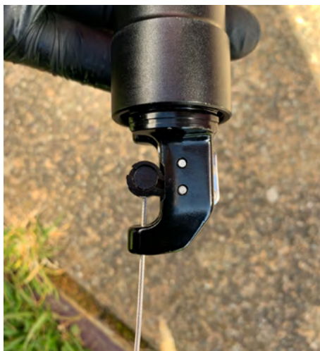
17. Insert the cable head into the dropper actuator.
