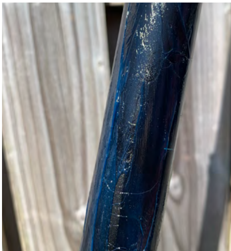
19. Apply grease to the outside of the seatpost.
