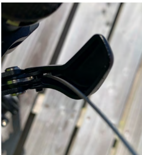
25. All the excess inner cable should now be sticking out of the lever and the outer cable should be in position. At this stage it is worth double checking your outer cable routing is good.
