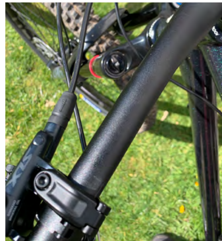
21. Carefully pull the outer cable and get it up close to the lever.
